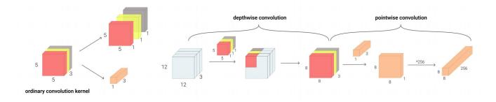
Fig. 4. Depthwise and pointwise convolution of MobileNet
